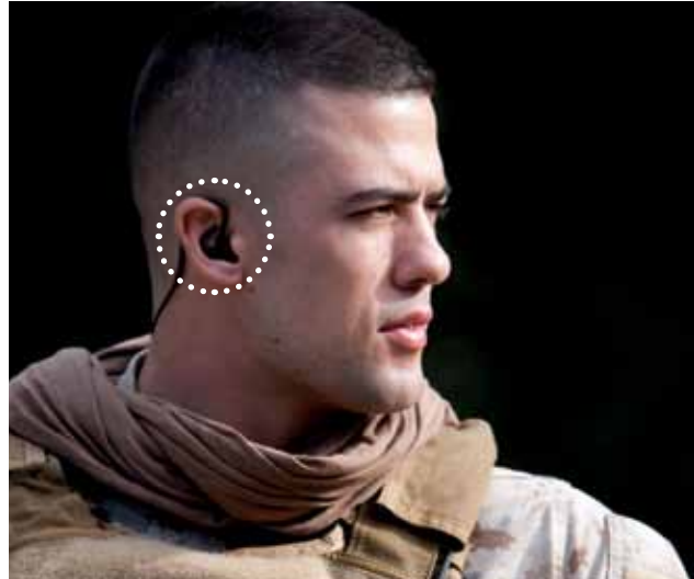
INVISIO's X5 headset, which sits in the ear, is discreet and comfortable. It can easily be used under a helmet, for example. The headset combines a speaker and a jawbone microphone (INVISIO Bone Conduction) in the same unit, does not pick up disruptive background noise, provides very good hearing protection, and can also amplify and reproduce background sound if required.
