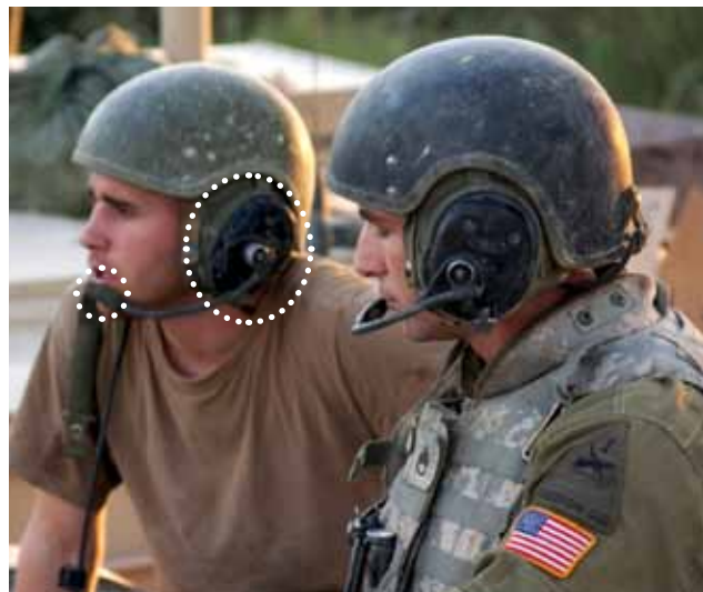
A large headset can cause strain on the neck and be uncomfortable to use for a longer period, as it presses against the head and becomes very warm. Hearing protection is not as effective as when it sits in the ear. The external microphone also picks up noise and disturbance, which makes communication more difficult.
